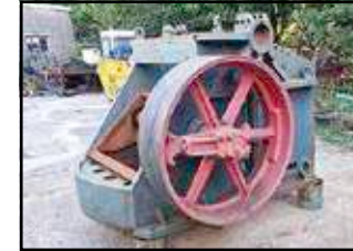
Undergoing refurb BROWN LENOX KUE KEN 36-10 Jaw crusher
