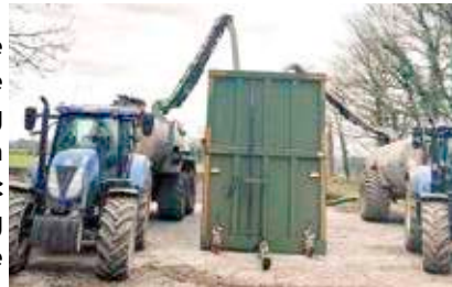
Mobile Sludge Holding Tank with hydraulic Lifting Axle
